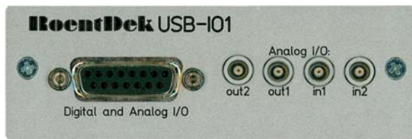
Figure: Front and rear panels of the USB-IO1 device with 2 LEMO analogue in-/output sockets, optional sub-D adapter (left picture), 5 digital input / 2 digital-output connections and the USB-port for the PC-connection.
