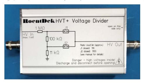
The **HVT+** voltage divider allows to downscale the effective voltage output by a factor of 10 or 100 (depending on jumper settings) so that very small voltages even below 1 V can be biased while the high voltage supply operates in its designated range of optimal stability.
