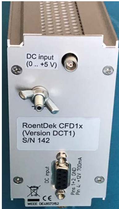
Figure 3.29b: CFD1x(+) with external input socket for positive signal or DC level input, here set for 0 – +5 V input range (left picture). The picture above shows the internal poti for the range adjustment. Do not change the setting without prior consultation with RoentDek .
