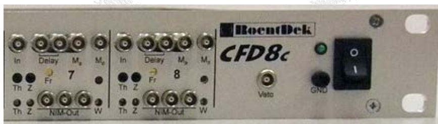
Figure 3.14b: Position of Veto input socket on the CFD8c front panel. For the CFD4c it is found on the rear panel
