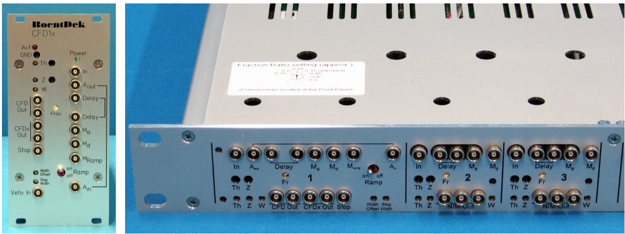
Figure 3.23b: CFD1x (left) and close-up of the CFD7x (right) showing the additional input/output sockets, switch and control potentiometers for the CFD x circuit
