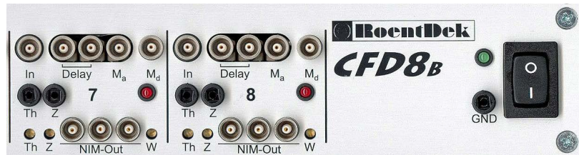
Figure 3.3b: Front panel inputs, test points and control potentiometers , not shown is the veto input and the CFD fraction potentiometer being on the front panel for c and x versions (see Figure 3.14b)
