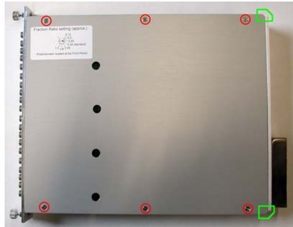
Figure 3.20b: Side panel of CFD4c with marked screws
