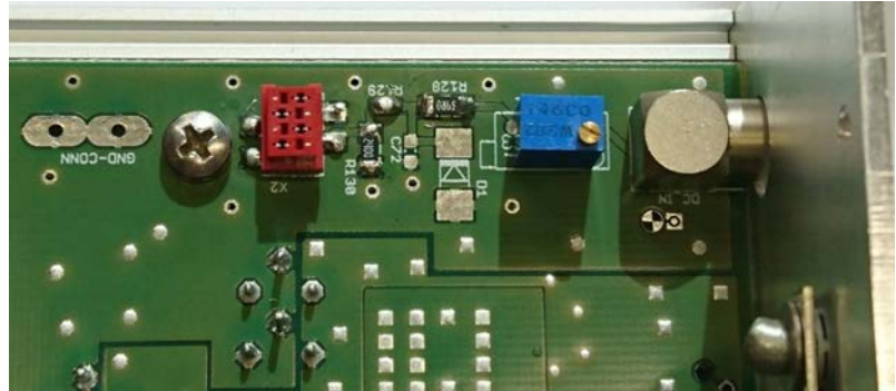
Figure 3.29b: CFD1x(+) with external input socket for positive signal or DC level input, here set for 0 – +5 V input range (left picture). The picture above shows the internal poti for the range adjustment. Do not change the setting without prior consultation with RoentDek .
