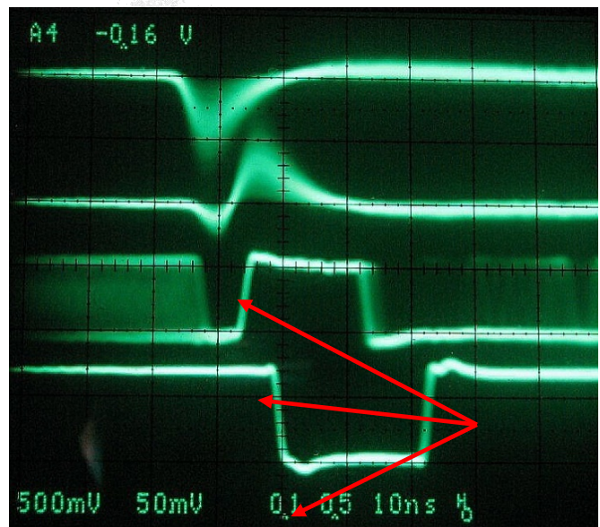
Figure 3.7b: Oscilloscope traces of in- and output signals of the CFD
