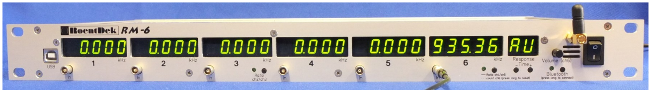
Figure: RM-6 counter module. Several displays allow simultaneous observation of up to six count rates.
