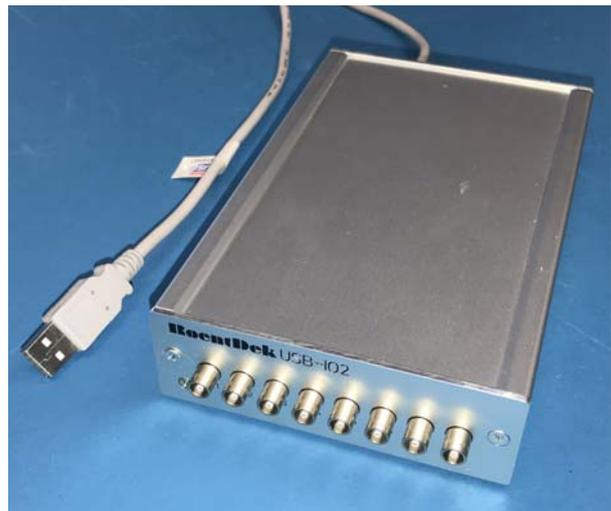
The software *USB-IO2\_GUI.exe* allows controlling up to 24 channels of 3 external (see figure above) or CFD-integrated **iUSB-IO2** units. The software recognizes each connected unit and will display the corresponding serial numbers according to the label on its case (for **iUSB-IO2** units the CFD serial number is relevant, the addressable voltage range limited from -25 mV to -2.5 V here, see figure below).
