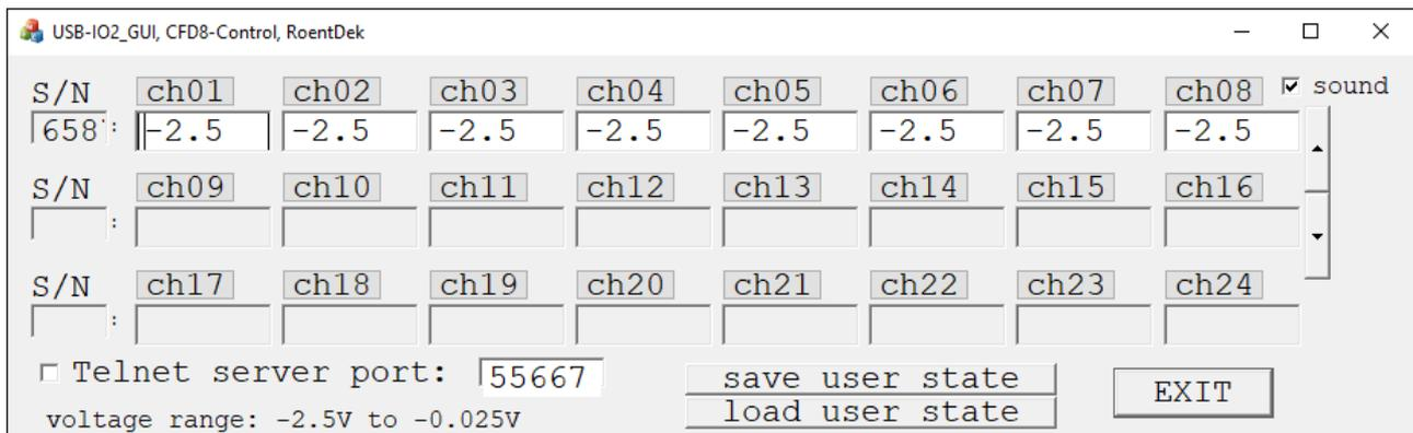
Set values can be stored in a file on disc and individually in an internal EPROM of any connected **USB-IO2** unit, also the last settings after program termination is automatically stored. Previously set or earlier-stored output levels will be maintained as long as the unit is powered. In case of CFD-integrated units the power state is determined by the main on/off switch on the CFD case. The internal unit will maintain the last setting even when the USB cable is removed.
