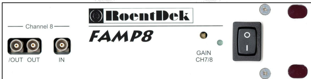
Figure 2: Detail of the FAMP8 front panel.
