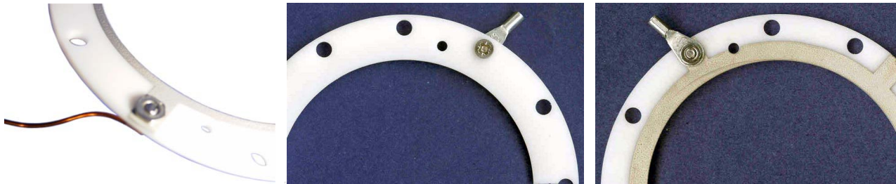
Figure 1.6: Cable connection on MCP ring. Left: cable clamped to a “front” ring without using a lug. Middle/right: cable clamped to a back ring with 3mm lug, countersunk M2 screw and special M2 nut.
