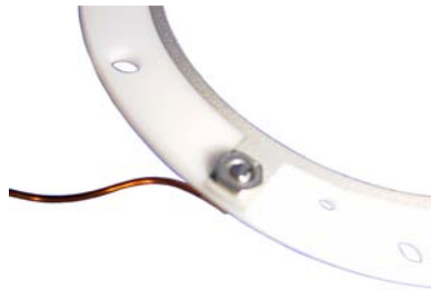
Figure 1.6: cable connection on MCP ring
