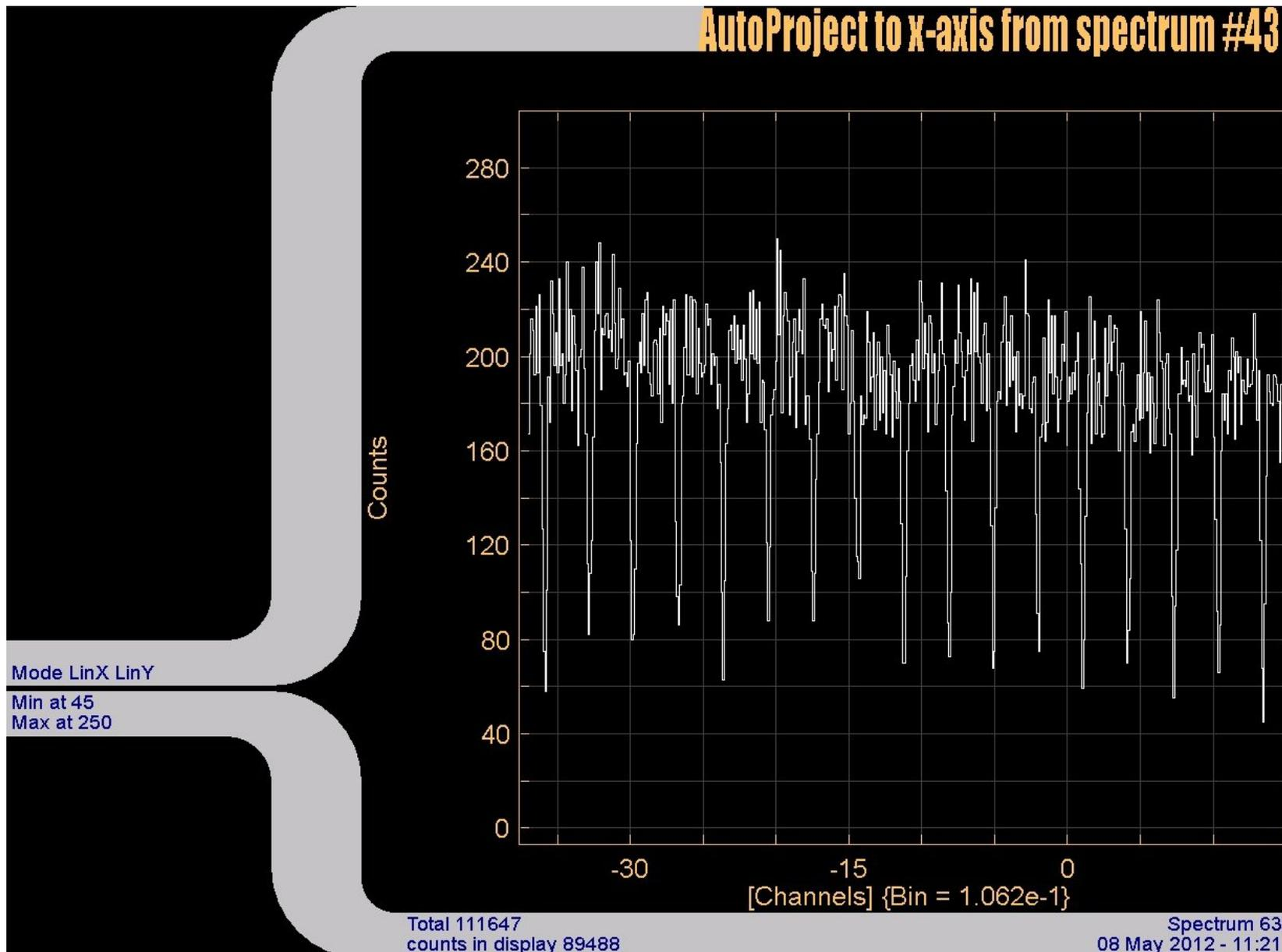
Line scan through the 0.2 mm obstacles of the mask's hexagonal structures. The bin size was chosen as 0.1 mm here, corresponding to 0.1 mm rms resolution (1500x1500 valid pixels) as can also be estimated from the data. We expect a resolution limit of < 50  $\mu\text{m}$ .
