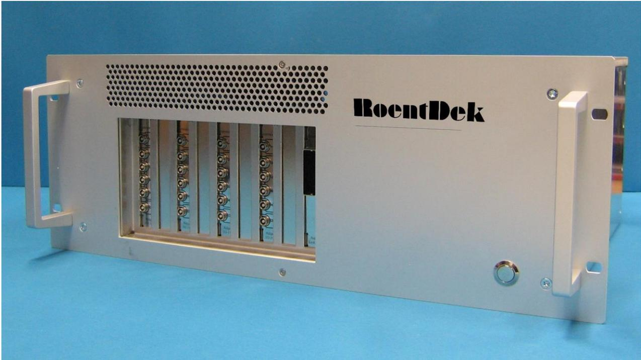
*Figure 2: the PCIe-extension crate can house up to 8 **RoentDek fADC4** modules (4 **fADC4** are displayed in this picture). An alternative version linking up to 5 **fADC4** and up to 2 **TDC8HP** is in development*
