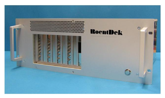
Figure 2: the PCIe-extension crate can house up to 8 **IROCHIDEK** fADC4 modules (4 fADC4 are displayed in this picture). An alternative version linking up to 5 fADC4 and up to 2 TDC8HP is in development
